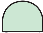
Excavation pleine section
